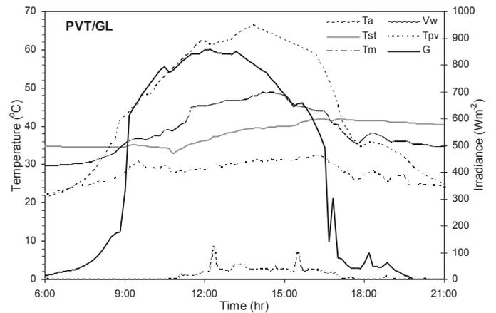
Fig. 4. Daily profile of temperatures, solar radiation and wind speed for the PVT/GL system with natural water flow operation
