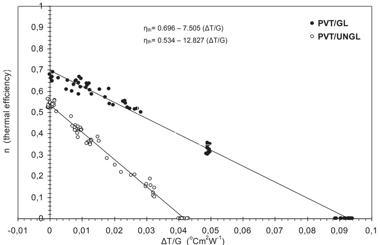
Fig. 2. Steady state thermal efficiency results of the studied PV/T models.
