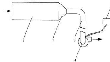
Fig. 4. Schematic diagram of the experimental setup; 1 – solar air heater, 2 – bell-shaped transition section, 3 – tube, 4 – centrifugal blower, 5 – frequency changer
