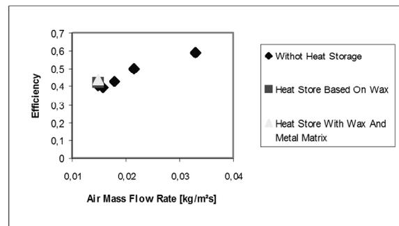
Fig. 6. The efficiency of the air heater with box-type absorber without heat storage unit as a function of air mass flow rate per unit area of the absorber. Average air heater efficiency of solar air heaters with heat storage units filled with wax and aluminum matrix structure and without aluminum matrix structure.
