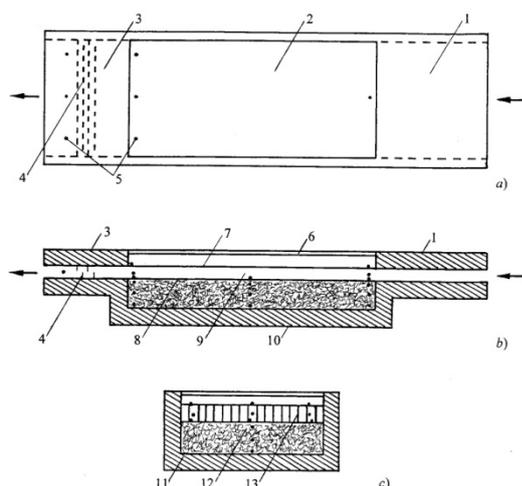
Fig. 1. Schematic presentation of solar air heater with box-type absorber and heat storage unit; 1 – inlet section, 2 – test section, 3 – outlet section, 4 – mixing section, 5 – thermocouples, 6 – glazing, 7 – top plate of box-type absorber, 8 – back plate of box-type absorber, 9 – collector channel, 10 – heat storage unit, 11 – insulation, 12 – paraffinic wax, 13 – slate
