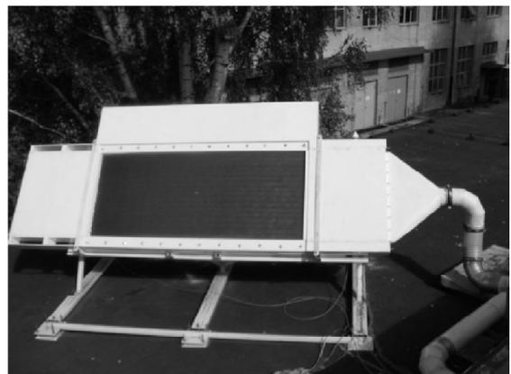
Figure 5 shows the investigated solar air heater with the heat storage unit.
