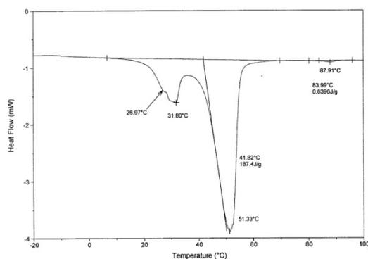
Fig. 2. DTA curve of paraffinic wax used in the experiment
