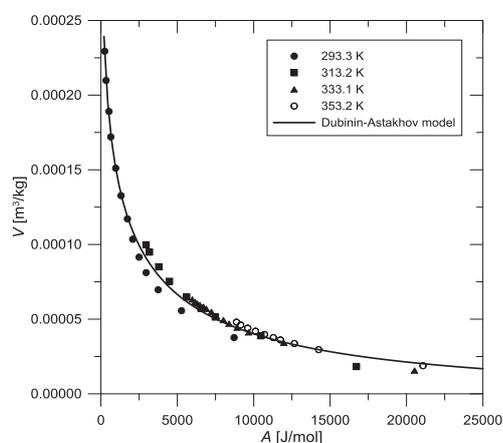
Fig. 1. Characteristic curve for water adsorbed on alumina
