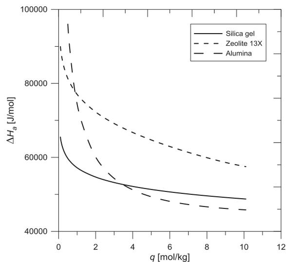
Fig. 10. Isosteric heat of adsorption of water on various adsorbents ( $T=298.15$  K)
