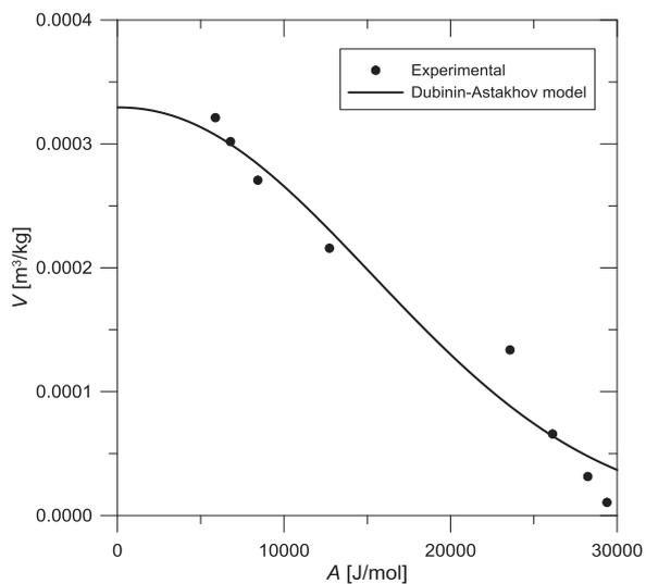
Fig. 7. Characteristic curve for ammonia adsorbed on polymer resin ( $T=298.15$  K)
