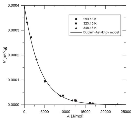
Fig. 2. Characteristic curve for water adsorbed on silica gel
