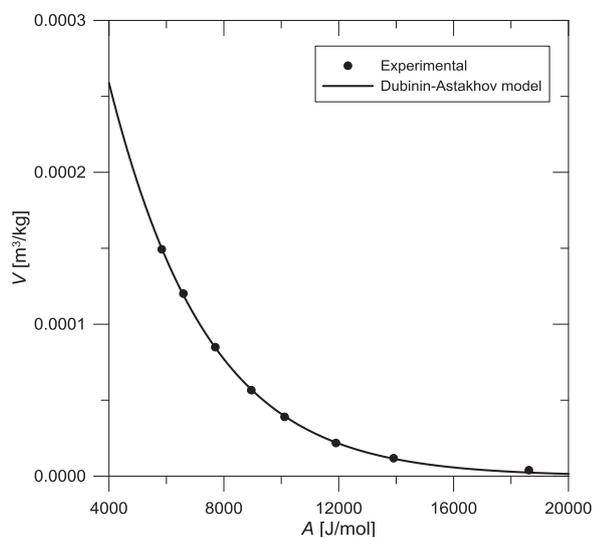
Fig. 5. Characteristic curve for ammonia adsorbed on charcoal ( $T=298.15$  K)
