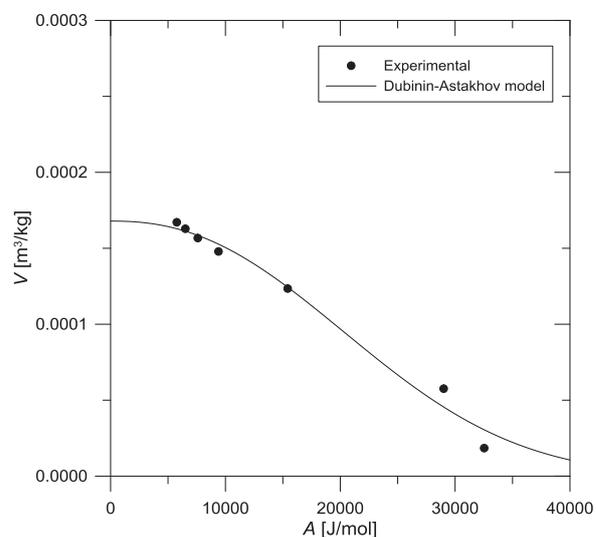
Fig. 6. Characteristic curve for ammonia adsorbed on clinoptilolite ( $T=298.15$  K)
