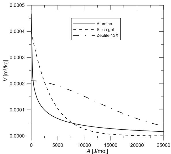
Fig. 8. Characteristic curve for water adsorbed on various adsorbents
