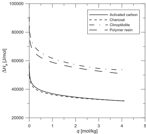
Fig. 11. Isosteric heat of adsorption of water on various adsorbents ( $T=298.15\text{ K}$ )
