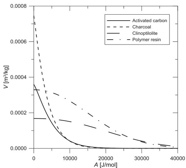
Fig. 9. Characteristic curve for ammonia adsorbed on various adsorbents
