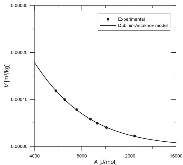
Fig. 4. Characteristic curve for ammonia adsorbed on activated carbon ( $T=298.15$  K)
