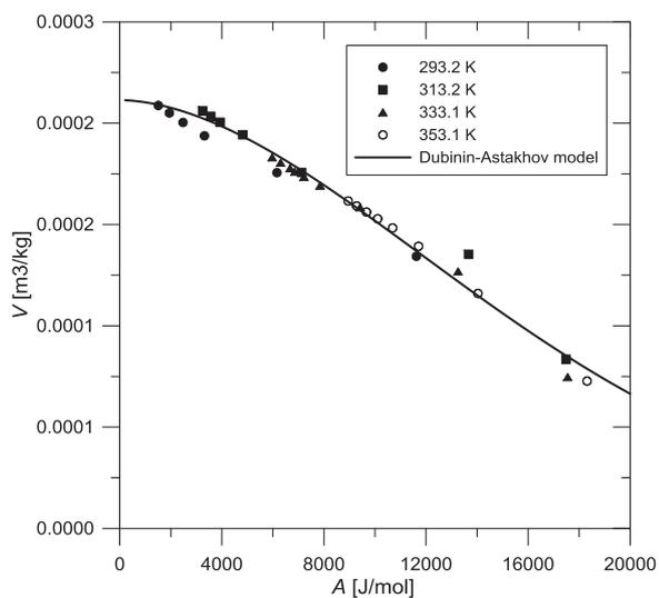
Fig. 3. Characteristic curve for water adsorbed on zeolite 13X
