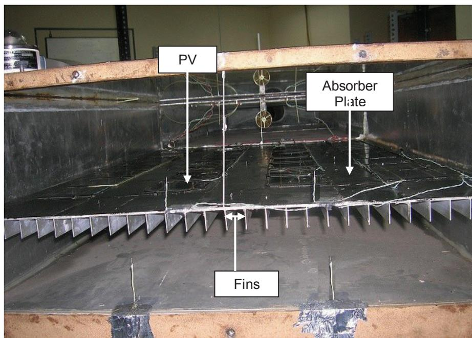
Fig.4. An example of the PV/T solar collector structure (M. Y. H. Othman, 2010)
