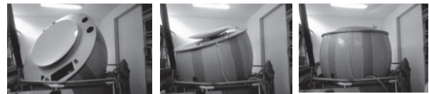
Fig. 8. Spherical shaped tracker tilting process. Starting from the left: 32 deg., 76 deg., 89 deg
