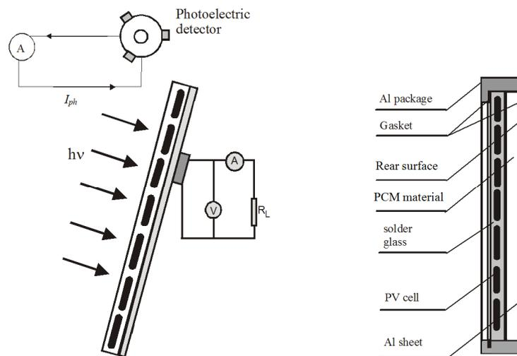
Fig. 4. The construction of tested PV/PCM system
