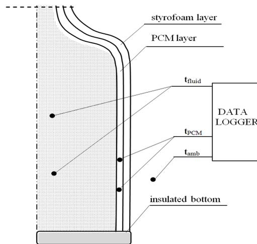
Fig. 2. The construction of tested double-wall bottle
