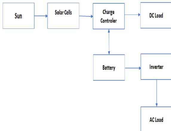
Figure 2. Basic working of a photovoltaic system
