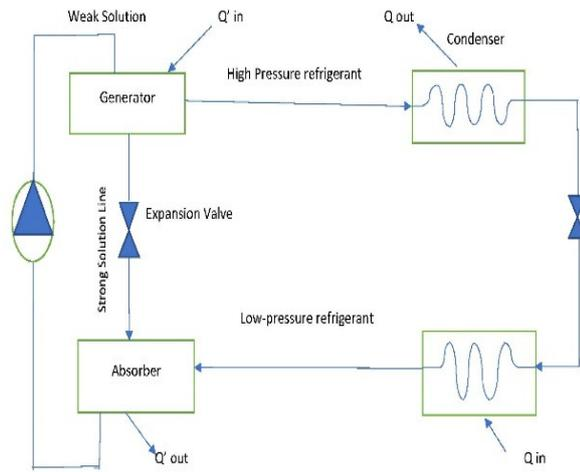
Figure 3. Basic Absorption system
