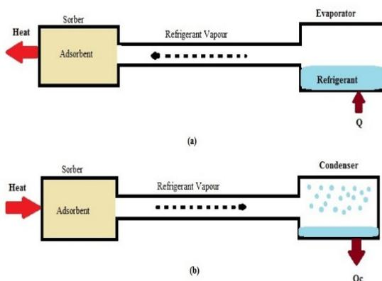
Figure 4. (a) The adsorption (Refrigeration) process and (b) The desorption (Regeneration) process
