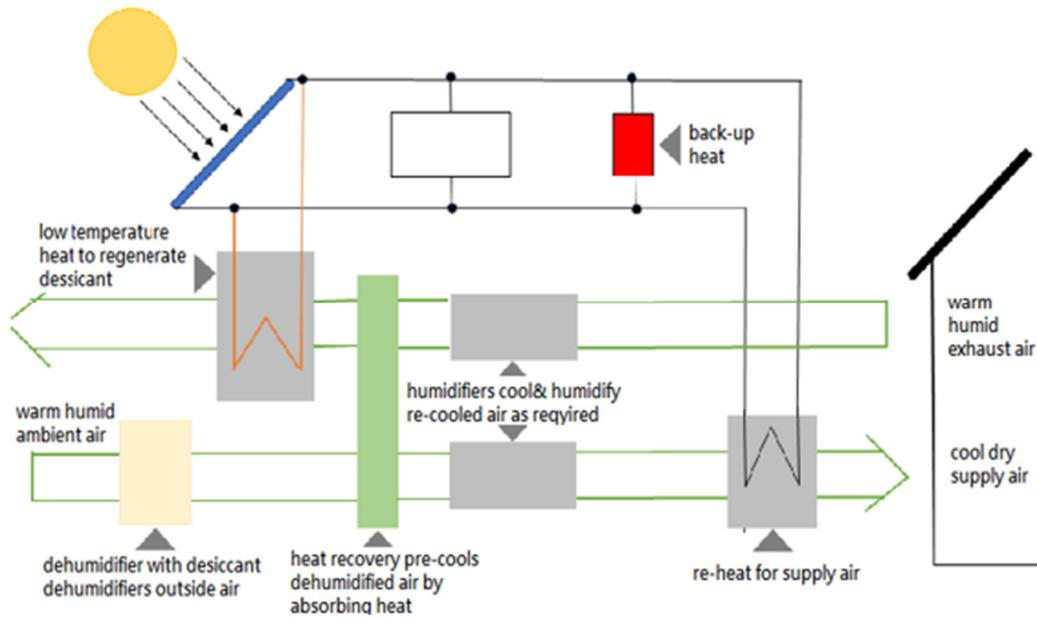
Fig. 5. Working of a desiccant cooling system.
