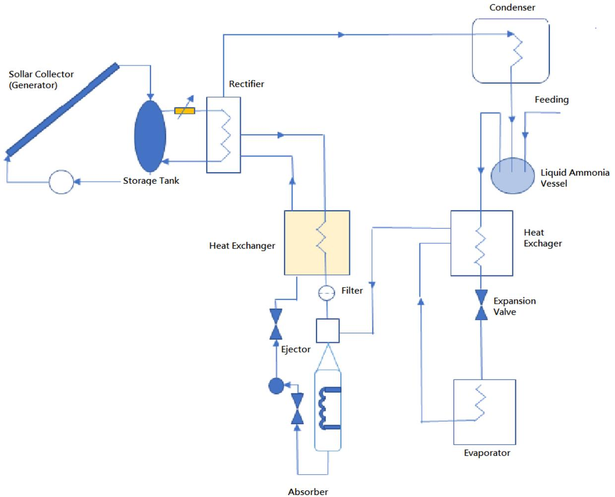
Fig. 3. Schematic diagram of an absorption system.
