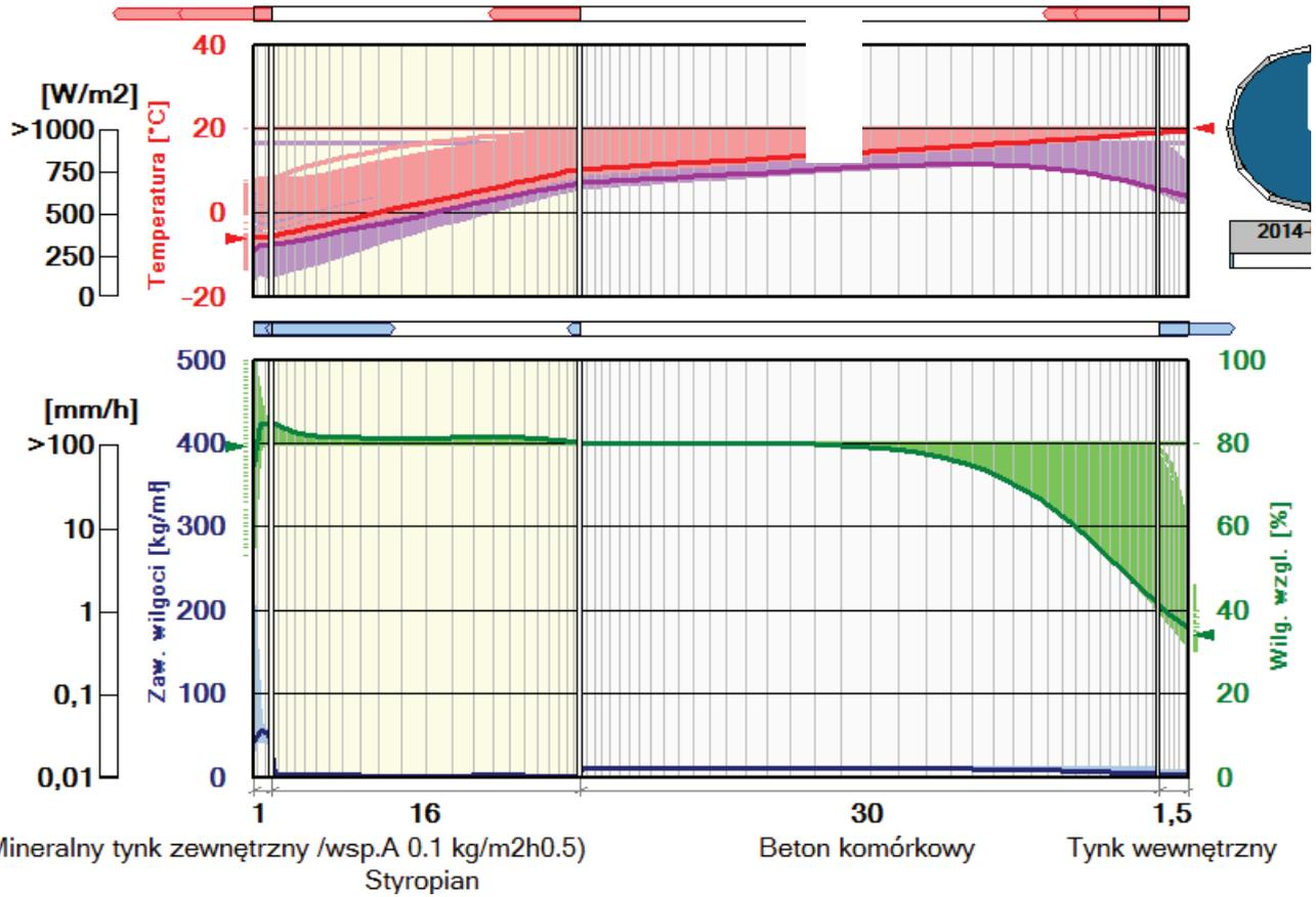
Fig.5. WUFI light simulation example showing how humidity can penetrate wall layers at different ambient temperature
